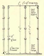
Fig. 207.—Wrought-iron pipe frame for switchboard.\*
